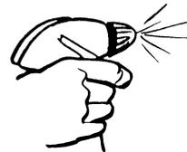
2. Wet film with slip solution to give slip for the squeegee.
