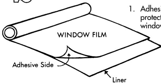
1. Adhesive surface is protected between window film and liner.
