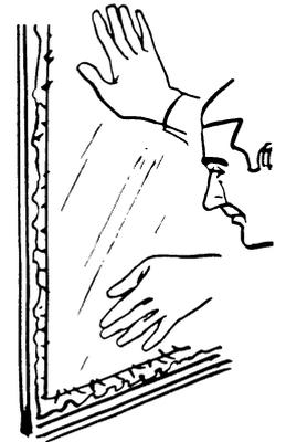
4. Position film by gently sliding on wet surface and smoothing out large air bubbles. Ensure all glass area is covered by film.
