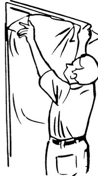
3. Carefully reverse film and line up straight edge at the top of the glass so that the adhesive side is now in contact with the glass.
